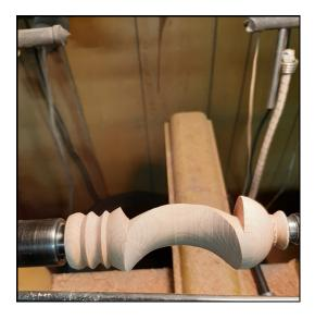
Once I am satisfied with the bottom, I turn back to finish the top, which is still secured by the tailstock. I cut off that extra bit, then turn that smooth. If I take light cuts, I find the Morse taper provides enough support. If you need it, Ruth's mandrel is threaded for a 1/4-20 drawbar through the headstock.
