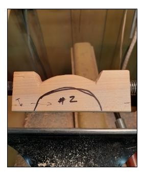
This is a good start on the shape. I still need to cut a bit farther, and increase the width of the cove slightly. It is still possible to go back to the #1 mounting position and cut more on the bead side if you think that will improve your shape.
