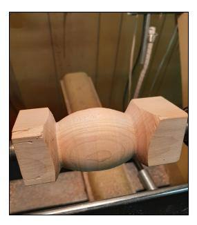
I'm going to take the blank from the position between points #1 and move to be mounted between the #2 points. It will still be parallel to the lathe bed, but now shifted the same 1/2'' of off-set in the other direction.
