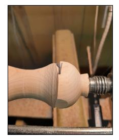
Now to round and add some design to the bottom of the handle where it will meet the bottle opener hardware.
