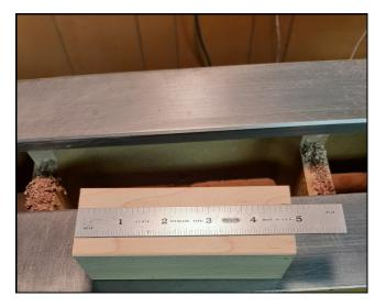
My blank for this project is a piece of hard maple. It is about five inches long and about 1-1/2" square. I have located and marked the center point on both ends. I also use a compass to mark a circle which will provide me with the off-set turning points. A circle about 1/2" from center is about right.
