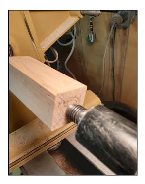
Now the fun part begins—the off-center turning. I remove the blank from the mandrel with the tap, and replace the mandrel with a drive center. I mount the blank between centers so that the #1 position on one end lines up with the #1 position on the other end. The blank should be parallel to the lathe. But shifted off-axis. My blank is about 1/2" from center, which is about right for this project. Even a small offset is quite obvious to your eye.
