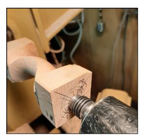
The rest of the project is standard spindle turning. I will finish the upper end of the handle, then turn a shape on the other end to match up with the bottle opener hardware.
