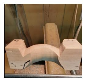
As the cove cut gets deeper, you will be getting closer to the lathe center axis, and your cuts will start to smooth out as you cut more wood and less air. Try to make the cove a nice sweep curve—again, less sanding later.
