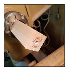
Now I am tapping the thread for the 3/8" bottle opener. The tap from Ruth is on a #2 morse taper mounted in the headstock. The tailstock live center helps keep alignment square. I spin the blank onto the tap a half turn or so, then advance the tailstock ram enough to keep the live center pin engaged. Keep going until the blank snugs against the shoulder of the tap. If it gets hard to turn along the way, I sometimes have to twist the blank off and apply a little wax to the tap threads.
