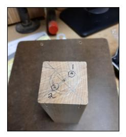
I made these off-center turning points, #1 and #2 on both ends of the blank. You want #1 and #2 to line up so that if you drilled a hole all the way through the blank it would pierce #1 on both ends. The blank will be shifted, but will always be parallel to the lathe axis.
