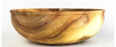
**Bronze Calabash Style Bowl**: Starting with the classic Egyptian calabash form we will turn and shape a piece of wood into a thin walled "Bronze metal" bowl. Key points are wood selection, thin wall turning with control, holding techniques to turn a true round bottom piece and much more. The use of reactive metallic paint and forced patination, along with the natural warping of a thin walled green wood vessel with create a stunning look when finished.
