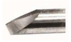
Look at your gouge from the side view and grind the high spots down and leave the low spots alone. Don't change the set-up angles.
