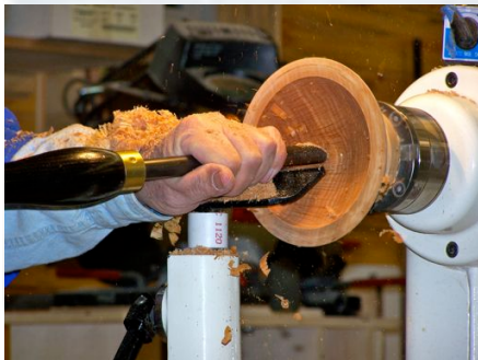
HOLLOWING THE TOP USING A BOWL GOUGE. THE INSIDE DOES NOT HAVE TO BE SANDED OR REFINED.
