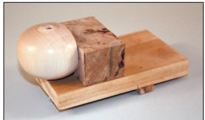
In this photo, the squaring block is used with a miter gauge to cut the second side off a body. Any square piece of wood would work. This really gives a different look, since you can see completely through the Christmas ornament.
