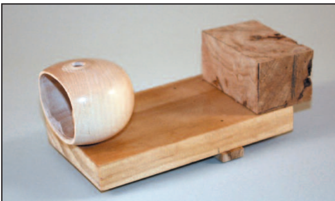
This photo shows the cutting sled that I made, and it is used with the miter gauge for my bandsaw. I use it to cut one or two sides off a body, giving a completely different look to an ornament.
